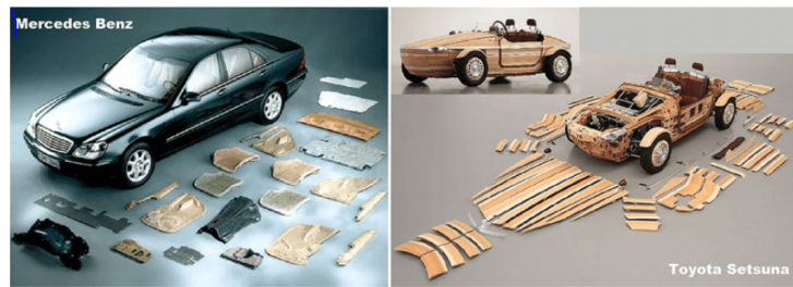
Figure 3 The different Automotive Components and parts that can fabricate directly from Natural fiber composite materials [15]
